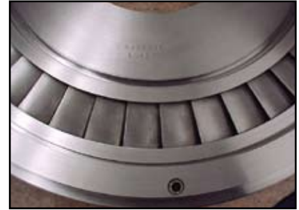
Steam turbine diaphragms
