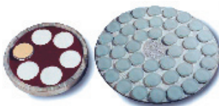
Workholder ring & working face of conditioning weight.
