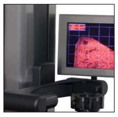
Exclusive software designed for multi-function measuring of many tool features rather than just simply measuring the length and diameter.
