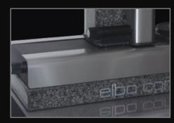
Base and column made of ground granite. The thermal inertia of this material allows the machine to be placed directly in the shop. Mechanical elements manufactured from stainless steel.
