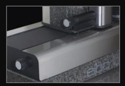
Micrometric registration of X and Z axes by means of two wheels which are essential for the collimation of the measure both with a fixed target function and in self-collimation.
