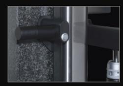
Manual axes movement. Axis unclamping by means of a single pneumatic control system. Approach speed controlled via software: 2 mm/sec.
