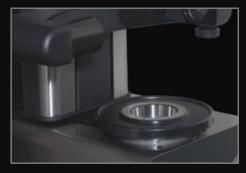
Interchangeable revolving spindle with mechanical rotation brake. Two preloaded ball cages allow a concentricity accuracy within 4  $\mu$ m.
