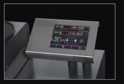
LCD touch panel display and software on a LINUX platform for a quick and easy operation of the machine and measuring functions.
